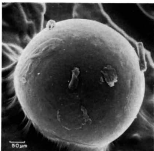
Fig. 3. Micrograph of etched silicon sphere.
